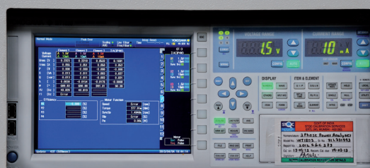
Efficiency determination as per IEC 60034-2-1 IS 15999 (Part 2 / Sec 1)
